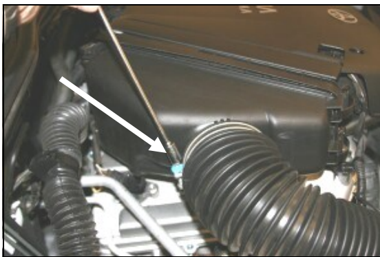
1. Disconnect the negative battery cable. Loosen the hose clamp on the factory intake tube where it connects to the airbox.
