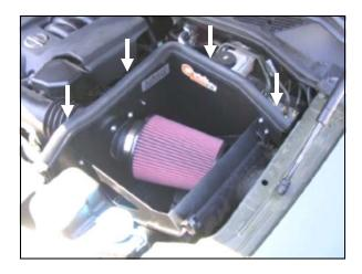
**10.** Install the Airaid Premium Filter (#1) onto the air filter adapter, and tighten the hose clamp. Install the weather strip (#5) onto the Quick Fit Panels as shown (*Note: Start at one corner and work your way around to the end to insure proper alignment of the weather strip*).
