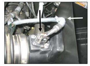
**9.** Reconnect the **MAF** sensor wiring harness to the sensor. Mount the factory wiring harness clip into the hole in the Airaid Quick Fit panel.
