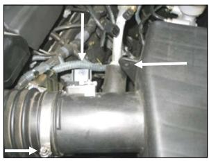
**1.** <u>Disconnect the negative battery cable.</u> Loosen the hose clamp on the factory intake tube. Disconnect the Mass Air Flow (MAF) sensor wiring harness from the sensor, and unclip the harness from the air box lid.
