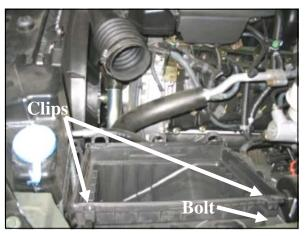
**2.** Unclip the factory air box lid from the factory air box base, and remove it from the engine compartment. Remove the factory air filter from the air box base. Using a 10mm socket, remove two bolts (three on some vehicles) from the air box base (save for reuse).
