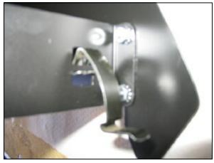
**7.** Remove the clip from the factory air box lid and install it in the Quick Fit Panels as shown.
