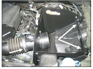
**8.** Install the Quick Fit Panel assembly onto the factory air box base using the factory clips. Slip the factory intake tube over the air filter adapter, and then tighten the factory hose clamp.
