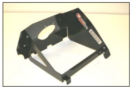
9. Assemble the Quick Fit Panels (#2&3) as shown, using the four supplied screws (#9), washers (#10), and nuts (#11). Apply the Airaid Foil Decal onto the Panel as shown.
