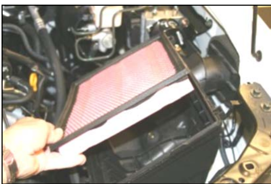
7. Remove the factory air filter.
