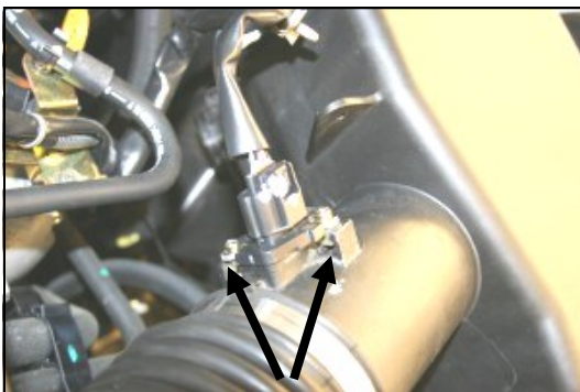
4. Remove the two screws that hold the Mass Air Flow sensor.
