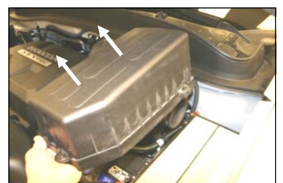
3. Remove the factory air cleaner lid from the vehicle.
