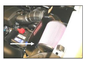
4. Remove the factory air filter from the vehicle.
