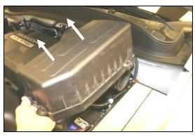
**3.** Remove the factory air cleaner lid from the vehicle.
