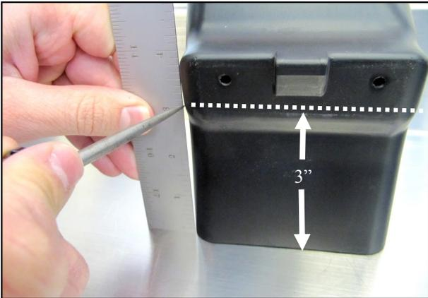
5. Set the factory air scoop on a workbench and mark all four corners at the three inch mark using a scratch awl. Using a straight edge and the awl, scribe a line connecting all four corners.
