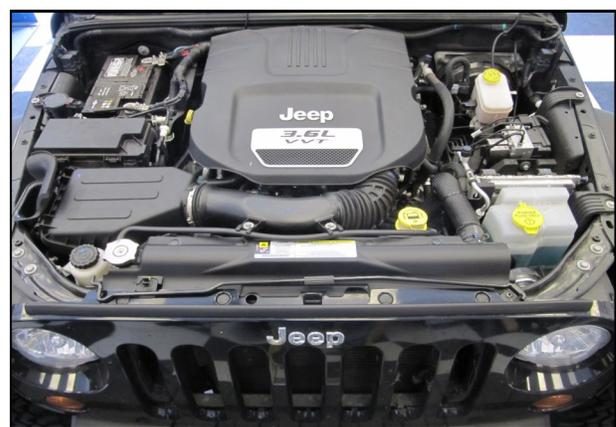
8. Install the Airaid Premium filter into the airbox and re assemble the intake system in the reverse order in which they were removed.
