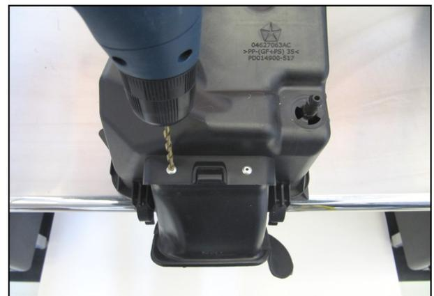
4. Drill out the rivet heads on the factory airbox and remove the air scoop. Remove any remaining rivet pieces from the air box and discard them.
