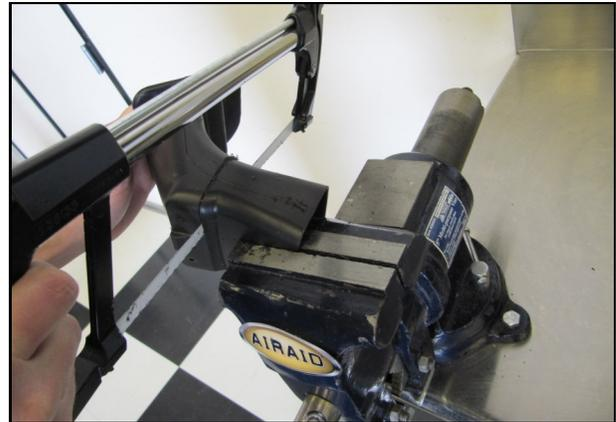
6. Firmly place the air scoop into a bench vice and cut along the line created in step 3 using a hack saw or equivalent.
