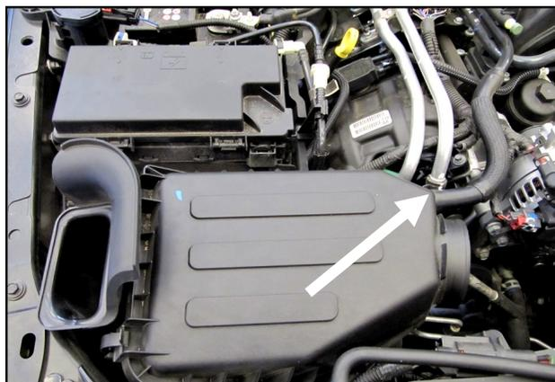
3. Disconnect the crankcase breather line in the top of the airbox. Remove the entire airbox as an assembly by unseating it from the mounting grommets in the inner fender and lifting upward.
