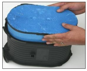
**3.** Remove the element from the filter housing and discard the element. Remove all remaining glue from the inside surface of the housing and clean surface using a rag.
