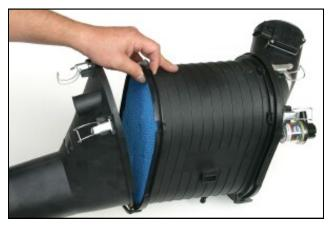
**1.** Remove the factory filter housing from the intake assembly by separating the inlet and outlet as shown above. Note: This step is performed in the vehicle. The vehicle is not shown in the pictures for added clarity.
