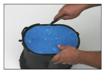
**2.** The air filter element is bonded to the housing on inlet side. Using a utility knife, carefully separate the filter element from the air filter housing as shown above. The utility knife will cut easily through the black glue that is used to bond the element to the housing. Use extra care to avoid personal injury from the sharp tool.
