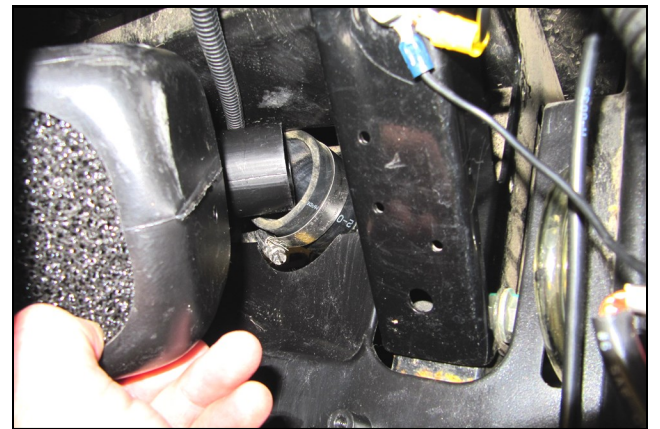
2. In the passenger side firewall area, locate the foam prefilter box and Loosen the hose clamp. Remove the prefilter box and set it aside.
