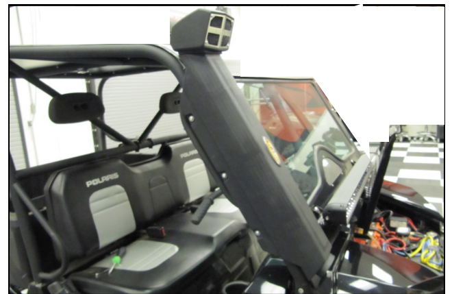
8. Outside view of properly placed Snorkel and clamps.
