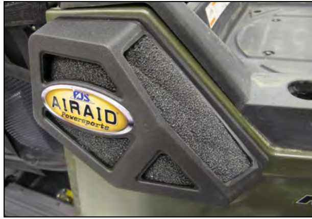
40. Insert the Foam Pre Filter (#6) into the Air Scoop as shown. Apply the Airaid decal as shown.
