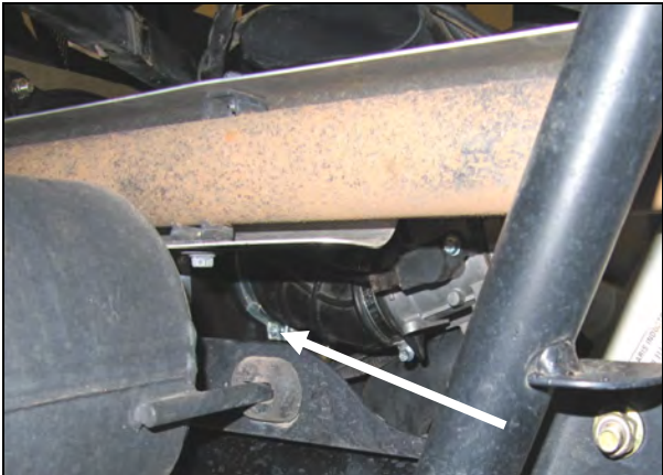
15. Loosen the large clamp on the factory intake tube
