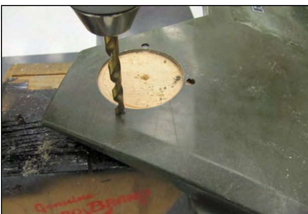
33. Drill 5/16" bolt holes in the Panel.
