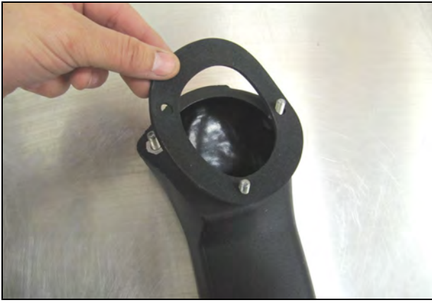
36. Slide the Riser Tube Gasket (#23) on to the Threaded Studs.
