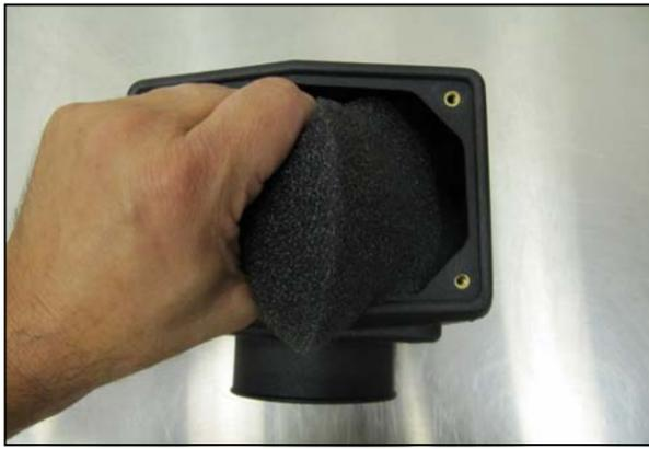
10. Insert the Foam Pre Filter (#6) into the Snorkel Inlet (#4).
