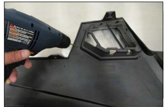
5. Using a drill and a 1/8" bit, drill out the four pilot holes in the inner fender.
