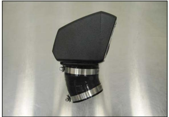
13. Install the Silicone Elbow (#7) and two #48 clamps onto the Inlet as shown. Leave the Hose Clamps loose for now.
