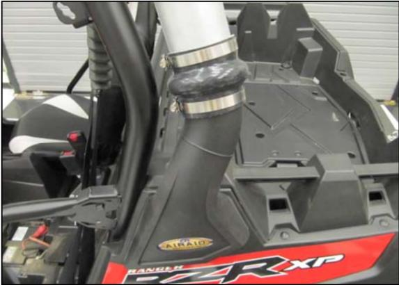
12. Install the Hump Hose (#8) and Aluminum Intake Tube (#3) onto the Fender adapter. Loosely install two #48 Clamps (#8) onto the Hump Hose.
