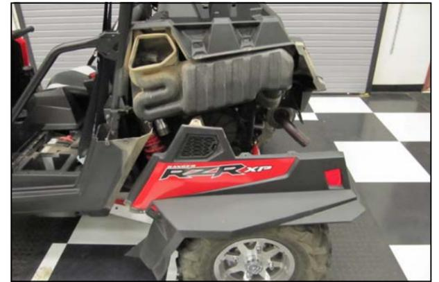
2. Starting on the Drivers side first, remove the nine T-27 head screws holding the fender in place. Remove the fender and place it on a work bench.
