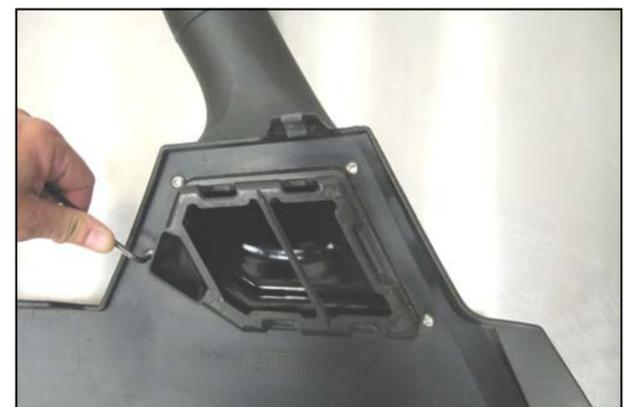
8. Attach the Fender Adapter to the outside of the factory Fender using four 1/4-20 button head screws (#14).
