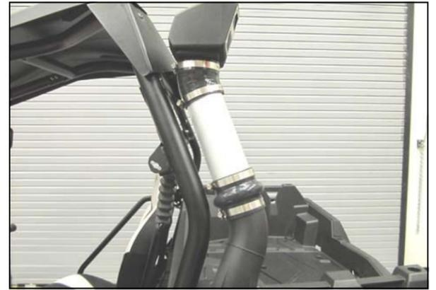
14. Install the Snorkel Inlet and elbow onto the Intake tube. Align the assembly into the desired position and tighten all of the Clamps. Repeat steps 2-14 on the Passenger side and re use the template, face down.
