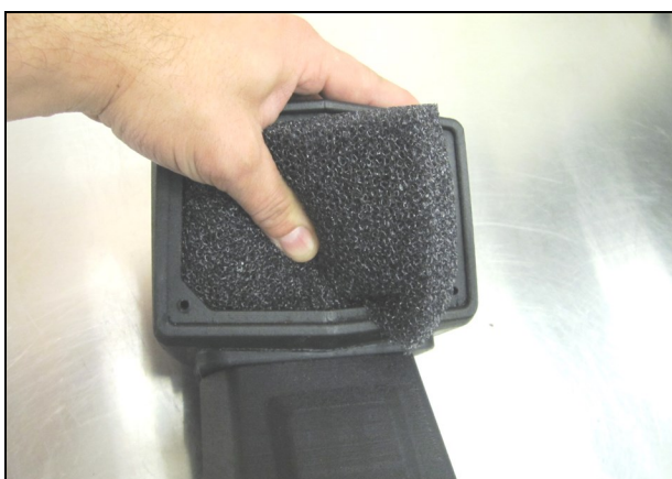
4. Carefully insert the Airaid Foam Prefilter (#7) into the Snorkel Inlet.
