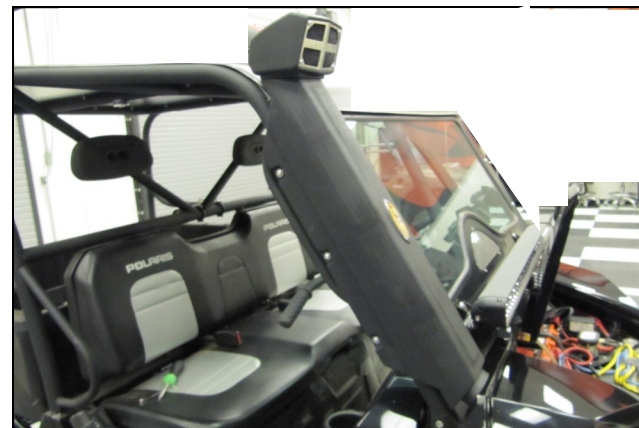
8. Outside view of properly placed Snorkel and clamps.
