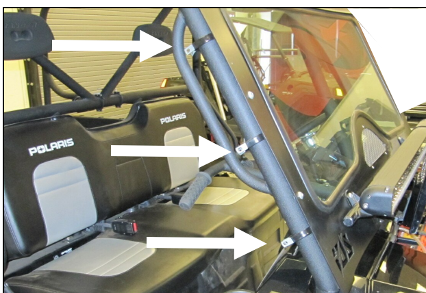
6. Preinstall the three Loop Clamps (#10) onto the right front A pillar of the cage.
