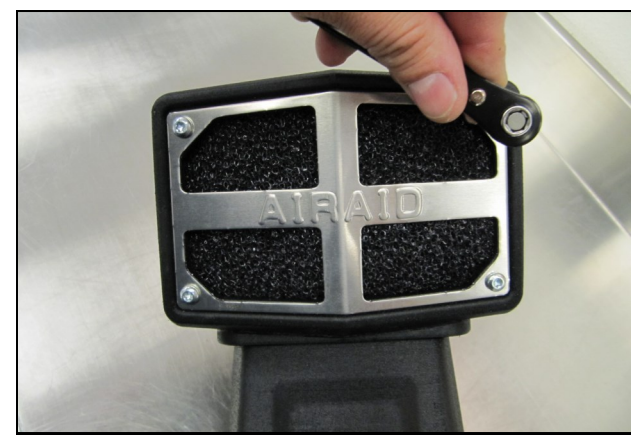
5. Install the Snorkel Screen (#4) onto the Inlet using the four 8-32 Button Head Screws(15).
