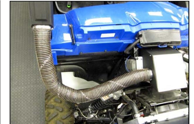
12. Full view of Duct routing. Duct is provided with an additional 8" in length and may be trimmed if desired.
