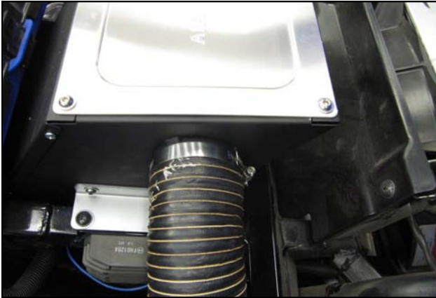
10. Install the Flexible Duct onto the Airaid performance airbox as shown. Re use the Clamp from step # 5.
