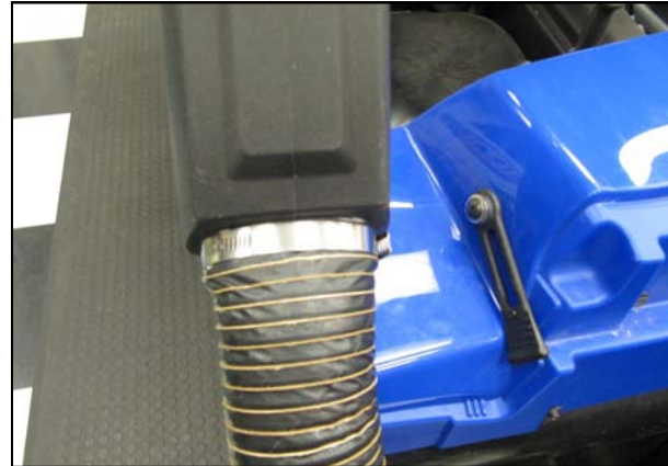
11. Install the other end of the Ducting onto the Snorkel tube using the #48 Hose Clamp (#16).
