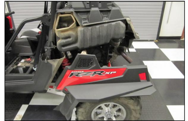
**2.** Starting on the Drivers side first, remove the nine T-27 Torx head screws holding the fender in place. Remove the fender and place it on a work bench.
