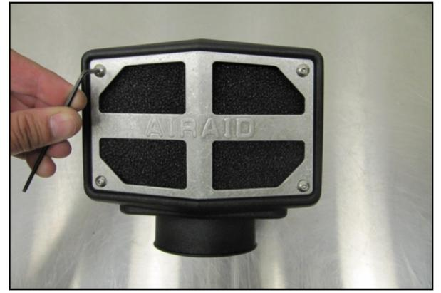
11. Install the Snorkel Screen (#4) onto the Inlet using four 8-32 Button Head Screws (#12) and a 5/32" Allen wrench.
