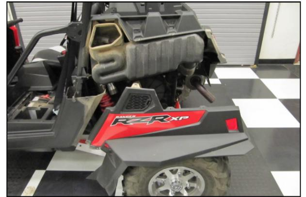
2. Remove the nine T-27 Torx head screws holding the fender in place. Remove the fender and place it on a work bench.
