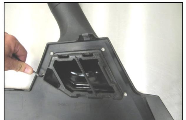
8. Attach the Fender Adapter to the outside of the factory Fender using four 1/4-20 button head screws (#13).
