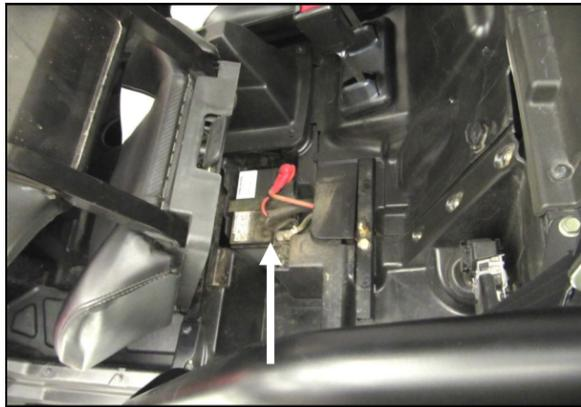
1. Place the range selector in Park and remove the seat from the vehicle. Disconnect the negative terminal on the battery.
