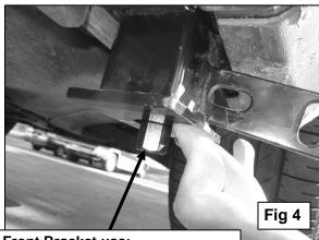
Front Bracket use: 12mm x 90mm Long Bolt Plate 12mm Flat Washer 12mm Lock Washer 12mm Long Coupling Hex Nut
