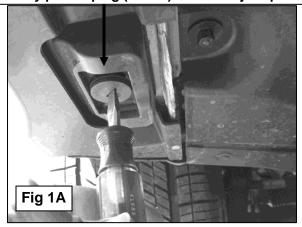
...or use a small screwdriver to pry up the push in factory plastic plug (center) and outer jack pad
