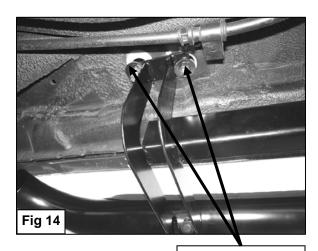
("U" Bolt) 10mm Hex Nuts 10mm Lock Washers 10mm Flat Washers
