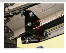
Mark and drill 7/16" Install 8mm revnut Remove the 8mm nuts, lock washers and lat washers from the running board.
