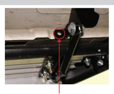
Drill 7/16" hole for 8mm rev nut
