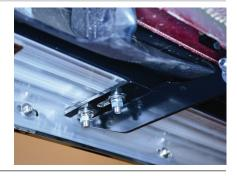
Adjust and level the running board, centering it between the front and rear wheel wells.
