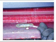
Place the front hanger bracket onto the vehicle and secure with an M8 flat washer, M8 lock washer and M8 hex bolt.
