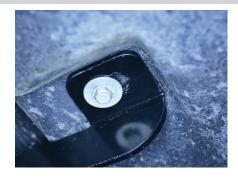
Locate and remove the rear hole plug. Insert an M12 T-bolt plate into the opening. Slide a plastic bolt retainer over the thread of the bolt to hold the bolt in place.
