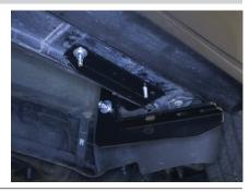
Place the L-shaped support bracket up to the unsecured end of the brace bracket. Secure with an 8mm hex nut, 8mm lock washer and 8mm flat washer. Snug the hardware, but do not fully tighten.
