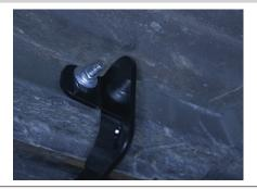
Place the support arm bracket onto the vehicle and secure with an 8mm hex nut, 8mm lock washer and 8mm flat washer.
