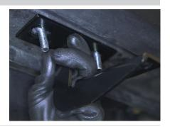
Remove the plug for the rear bracket rocker panel mount location and install a 48mm tab T-bolt and plastic retainer.
