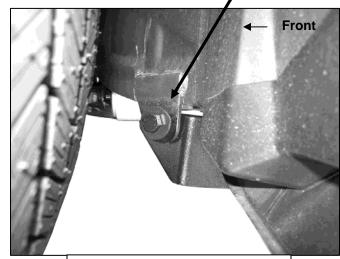
(Fig 3) Driver side tied down loop pictured from behind front tire
