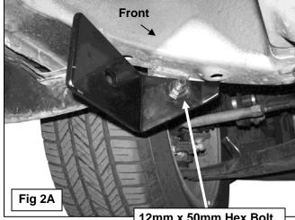
12mm x 50mm Hex Bolt 12mm Lock Washer (2) 12mm Flat Washers 12mm Hex Nut
