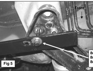
8mm x 60mm Hex Bolt 8mm Lock Washer 8mm Flat Washer
