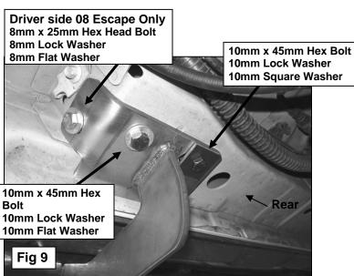
09-010 models-Install passenger side rear Mounting Bracket between exhaust support and body panel. Secure with factory hex bolts
