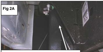
Install mounting bracket with (1)12mm x 120mm Hex bolt (1)12mm x 440D flat washer (1)12mm lock washer
