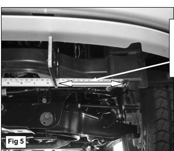
Measure from the mounting point for the splash guard to the bracket on the driver and passenger sides. Use this measurement as a reference point to check location before cutting the 1/2" wide x 4" long slot
