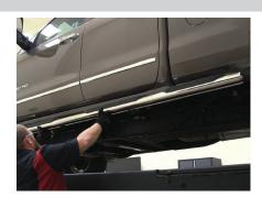
Attach the side bar to the brackets with six of the 10mm hex bolts, locking washers and flat washers.
