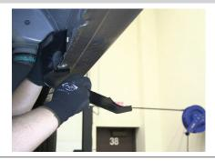
Locate the fourth tab location from step 1 and remove the upper and lower rubber plug from the access hole.
