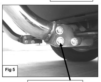
12mm x 30mm Hex Head Bolts 12mm Nylock Nuts 12mm Flat Washers
