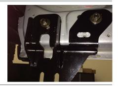
If your vehicle is not equipped with lower threaded inserts: Rotate the 12mm bolt plate until the 10mm nut lines up with the bottom mounting hole. Secure the bottom of the bracket with a 10mm hex bolt, lock washer and flat washer.
