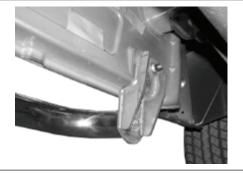
On the driver-side front location remove the factory tape covering the mounting slots in the rocker panel.
