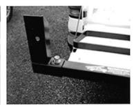
place Backrack c/w Railmount Bracket on to Rail Plate and secure to Stake Pocket Bolt
