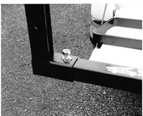
place Backrack c/w Toolbox Brackets on to bed rail and secure to stake pocket bolts.
