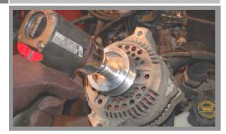
Remove the alternator mounting bolts, lift the alternator out of its cradle to access the pulley.
