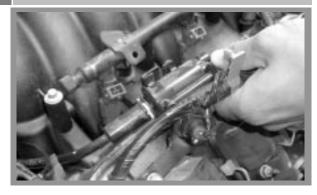
Unclip the purge solenoid from the intake manifold. Release its vacuum tube from the manifold be gently prying the retaining collar upwards with a flat head screwdriver while pulling.
