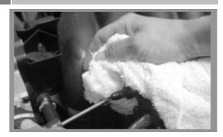
Carefully release any fuel system pressure by removing the cap at the front end of the driver side fuel rail and depressing the Schrader valve using a small screwdriver while shrouding the valve with a rag or cloth.
