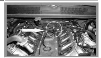
Reach behind the intake manifold and unplug the oil pressure sending unit (shown circle in photo).
