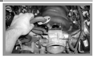
Using a 10mm socket, remove the throttle body bracket and EGR tube from the front of the intake manifold.
