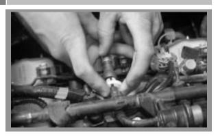
Using the 3/8" spring lock tool, disconnect the fuel rail feed hose.
