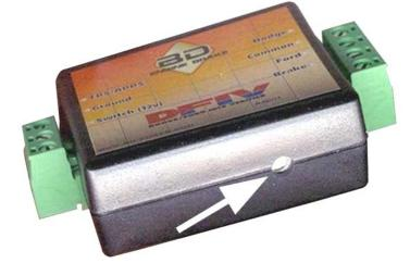
With the throttle at idle, start the engine and turn on brake switch. Then, using a small flat bladed screwdriver, turn the small adjusting screw in the DFIV Module counterclockwise or clockwise until the test light JUST turns on.
