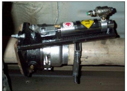
Install the rear exhaust with the adapter flange onto the mounted BD Brake valve, then install the v-style wedge clamp and tighten it.
