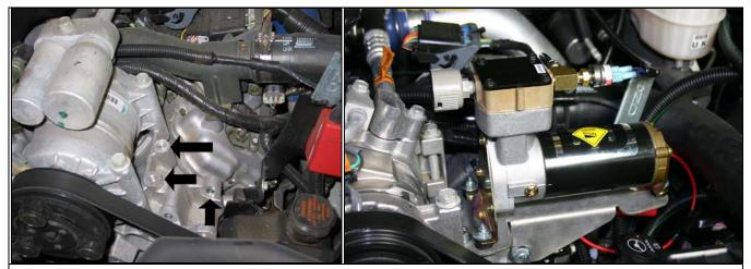
Locate a position by the air conditioner compressor to mount the pump assembly. There should be two open ended threaded bolt holes that will accommodate the two rear mounts of the air compressor nicely.
