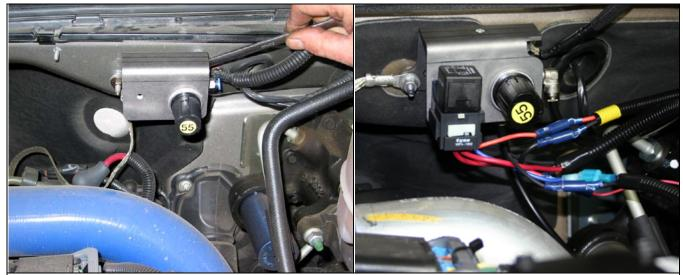
Locate a spot just to the left of the brake master cylinder assembly and install regulator & relay assembly. You may have to remove the relay and the relay socket holder to enable access to the mounting screw.
