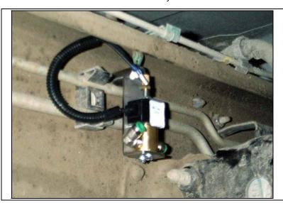
Using the hardware provided, mount the Solenoid Valve Assembly to the inside of the frame rail and reinstall filter.
