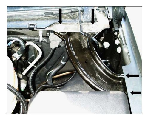
Locate the four (4) mounting bolts that secure the driver's side fender brace and remove them.
