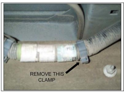
There is a wiring harness running along the outside of the driver's side frame rail and is secured with plastic clamps.
