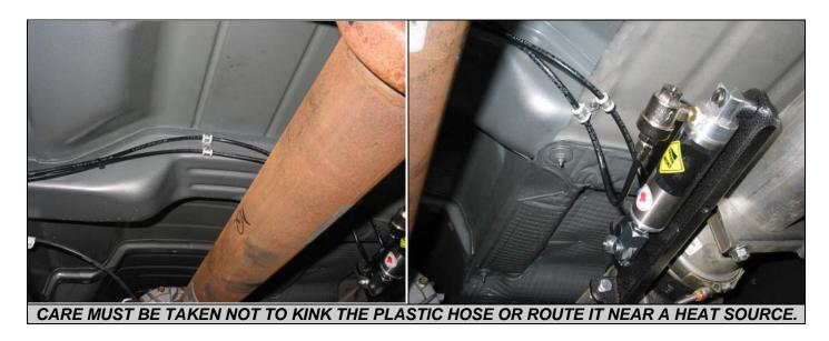
Insert one end of the remaining ¼" hose into the straight fitting of the solenoid valve and route this hose as well as the plastic hose with the yellow snorkel filter along the frame rail and into the engine compartment. The hose from the solenoid valve will later be attached to the regulator on the air compressor assembly when that is installed. The hose with the filter can be run through the firewall and secured under the dash area, away from any moving or heated equipment.
