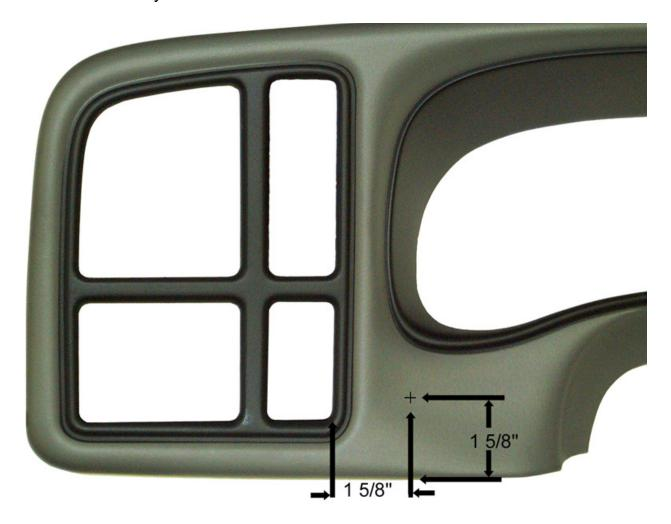
Note: This measurement must be exact as possible to ensure room for the switch on the inside of the panel.
