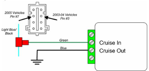
NOTE: For this change, the firmware loaded inside the Exhaust Brake Controller will have to be at least version 1.30. There is a version identifier sticker on the back of the module if you are unsure which version you have.
