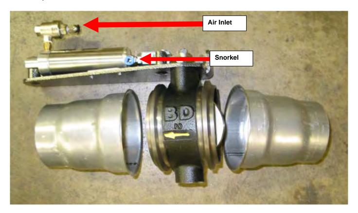
You must next run the snorkel line from the exhaust brake cylinder to underneath the hood of the vehicle in a dry clean area. You should see this connection on the front end of the exhaust brake air cylinder.
