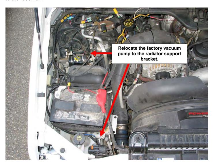
Remove the electric vacuum pump from the stock mount and re-install onto the new relocation mount provided. Trim the rubber ends on the three vibration dampers to
