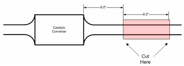
Slide the supplied flanges over the each side of the cut exhaust. The flange closest to the front of the vehicle will need to be welded. A good clean weld is needed to
