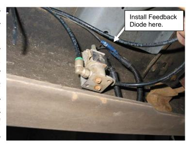
At the same time it is probably a good idea to install the Feedback Diode assembly. Just connect the quick connectors together matching Black to Black (Ground) and Red to power.
