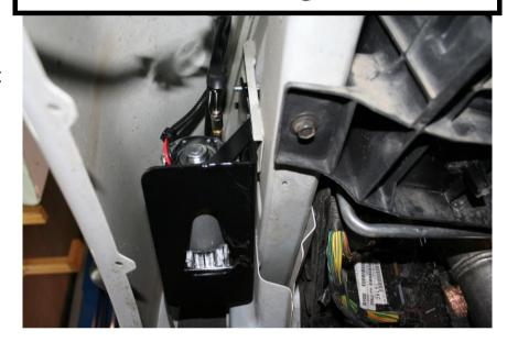
Tighten all bolts to secure the assembly. Route the compressor hoses & wiring harness up through the body opening at the rear of the battery. They will be hooked up later.
