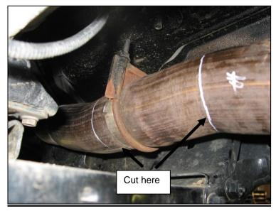
Insert the exhaust brake and secure with supplied 'V' band clamps. Be sure that the air cylinder bracket extends toward the rear of the vehicle
