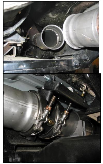
Ensure the exhaust brake and rear exhaust sections are pushed all the way forward on the front pipe so that the front adapter flange is up against the stop that is on top of the front pipe section then WELD the front adapter in place. Install the rear adapter to the pipe using the supplied band clamp.
