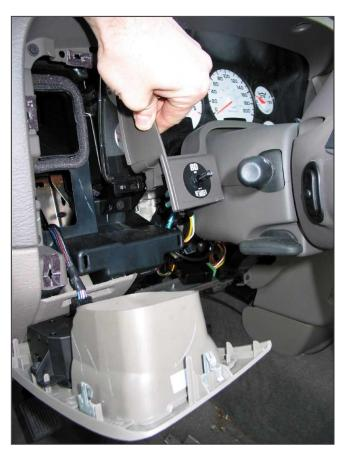
Install the switch into the drilled hole and secure it with the plastic lock ring. Reinstall the dash trim panels by reversing the removal procedure.
