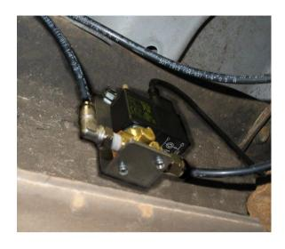
NOTE: To remove the plastic hose from the quick-connect coupler, push the outer ring toward the fitting and pull the hose out.
