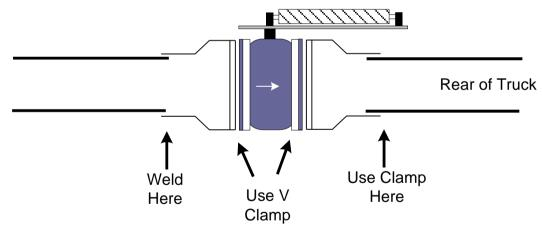
**NOTE:** SECURING THE FRONT ADAPTER WITH JUST A CLAMP WILL CAUSE LEAKAGE AND NOT ALLOW THE BRAKE TO OBTAIN FULL BRAKING PRESSURE.
