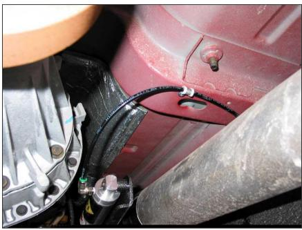
As indicated by the photo, secure the plastic hose by installing the clamps provided to the body of the cab. Drill a 1/8" pilot hole in the cab body as shown in the photo and secure the anchor clamps with the provided self-tapping screw.
