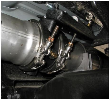
Tighten all mounting nuts and bolts that secure the brake to the flanges.
