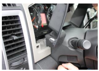
Install switch into drilled hole and secure with lock ring then reinstall dash trim panels by reversing the removal procedure.
