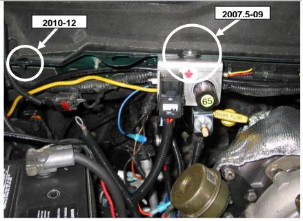
Install the regulator assembly underneath the hole (shown on figure to the right). The lock washer and flat washer should be installed on top of the plastic cowling with the Phillips screw holding everything in place.
