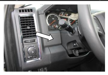
Remove the three screws holding the insert into the dash; gently pull the insert toward you.
