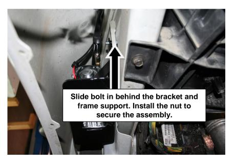
Tighten all bolts and secure assembly. Route the compressor pigtail wiring harness up towards the regulator assembly you previously installed. You will also need to route a small section of plastic air hose from the quick connect of the air compressor outlet to the regulator assembly.
