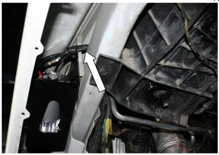
Use the wiring diagram on page 19 as a reference for the wiring of the air hoses and the electrical wiring. NOTE: Be sure to keep all hoses and wiring harnesses away from any moving parts or heat sources.
