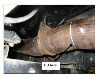
Insert the exhaust brake install with supplied 'V' band clamps. Be sure that the air cylinder bracket extends toward the rear of the vehicle.
