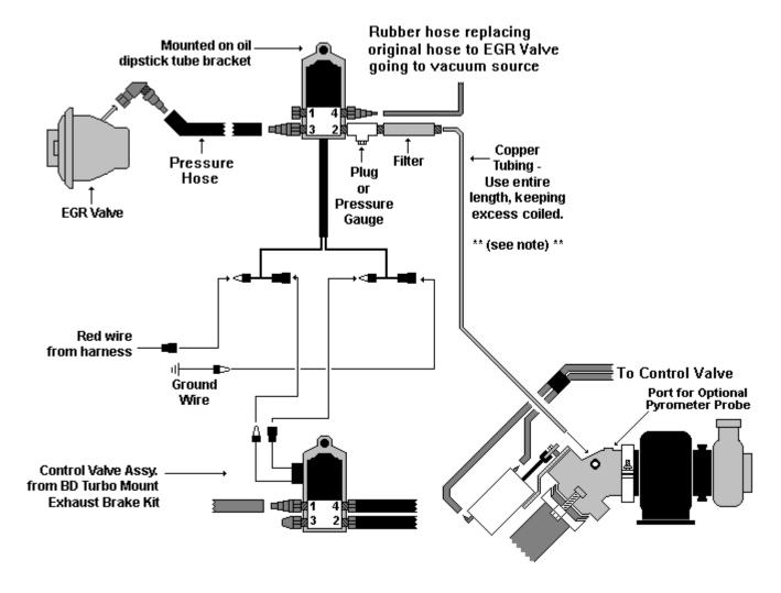
\*\*NOTE\*\*: Ensure that the copper tubing is properly secured to prevent breakage.
