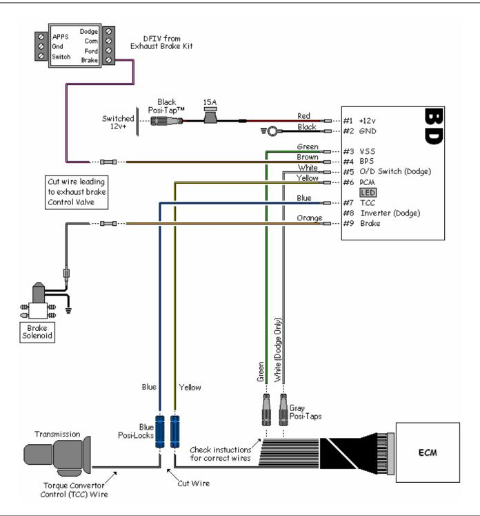
**ATTENTION:** Use this wiring diagram for 1999-2005 Dodge vehicles if you want the exhaust brake to be controlled by the AutoLoc module.
