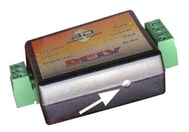
small adjusting screw in the DFIV Module counterclockwise or clockwise until the test light JUST turns on.
