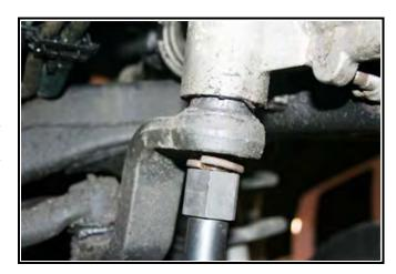
Slide support bar into place, where the mounting feet are positioned in between the sway bar mounting and the frame.
