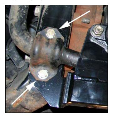
Ensure free movement (rotation) of the steering box sector shaft nut. If not free moving undo sway bar bolts and readjust.
