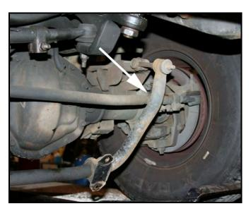
The 1-5/16" socket will be required to remove the steering box sector shaft bolt with lock washer. Retain the lock washer for re-installation with new nut.
