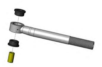
Locate the driver's side track bar section (#1302030-1). Thread the straight grease nipple (#1302057) into thread port on the side of the unit.
