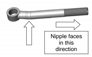
Open the bag of poly bushings (#1302033). With the supplied grease rub it all around each half of the bushing (ID and OD). Once fully lubed press the each half of the bushing into the track bar ends. Finally lube the steel sleeve and press into the bushings.
