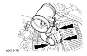
3. Connect Inlet Hose (straight end hose #1302191) to valve cover breather port. Secure this connection with a #32 spring clamp (#1302197).
