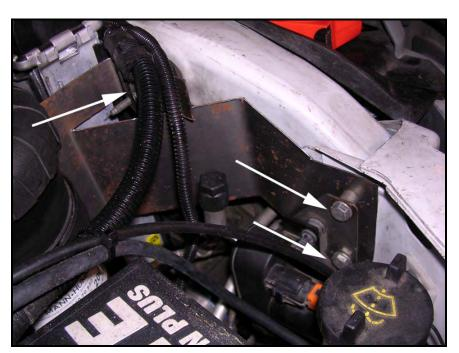
6. Install CCV filter onto the bracket (#1302180) using the provided 5/16" hardware. Then assembly into vehicle with the bolts removed from radiator support.
