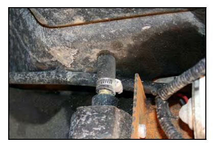
12. Install the drain hose from the bottom of CCV Bottle through the hole in the fender liner.
