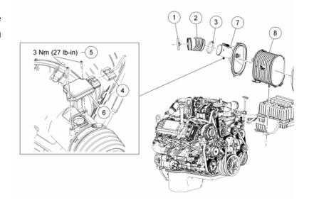
2. Remove the turbo air inlet hose and snorkel.
