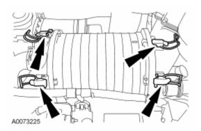
1. Remove the turbocharger air intake plastic pipe, and the air filter box from the vehicle.
