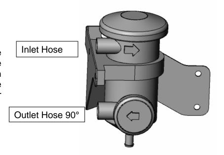
7. nstall the Outlet Hose (bent hose ends 90°) to the bottom (Outlet) of the CCV Bottle with a spring clamp #32.
