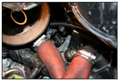
4. Re-install the turbo inlet tube, with hose attached. Be sure no kinks are formed.
