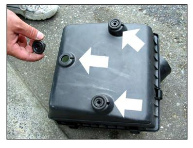
Remove the rubber stands/grommets from the bottom of the OEM airbox.
