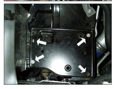
Remove four (4) bolts securing the airbox tray in place.
