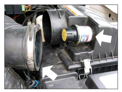
Remove the air inlet hose from the airbox.
