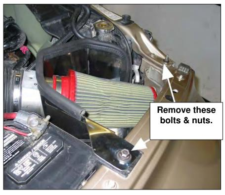
Remove the airbox retaining nut and lift the airbox off of the support stand to remove.
