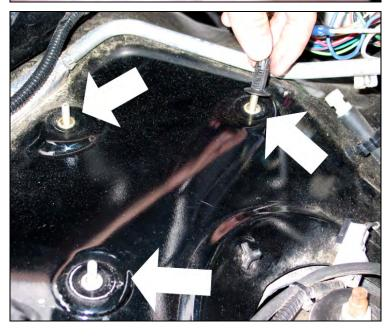
Place the stands on the mounting bolts in the fender.
