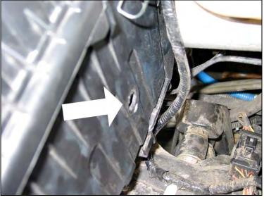
On the firewall side of the OEM airbox, there is an Intake Air Temperature (IAT) Sensor. Twist and remove it from the airbox.
