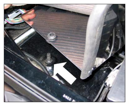
Line up the grommets on the base of the X-Intake Airbox with the stands on the fender and push down ensuring the base is secure on the mount stands.
