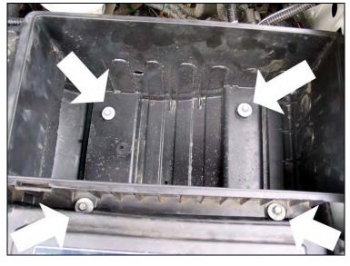
Remove the OEM air filter and then remove the four (4) mounting bolts that hold the OEM airbox in place.
