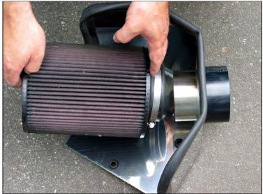
Follow the manufacturer's instructions to prepare the air filter element and then install it on X-Intake Airbox housing (as shown in the picture to the left) and secure with the filter hose clamp.
