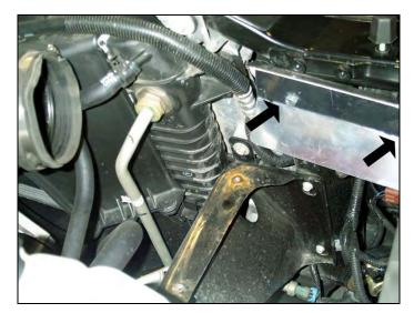
Install the splash shield supplied in the kit to the front support and secure with the bolt provided.
