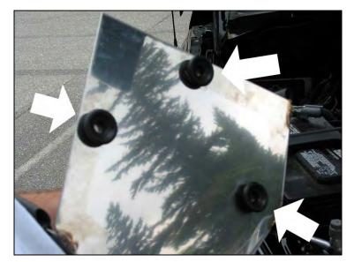
Install the grommets into the holes on the bottom of the X-Intake Airbox.
