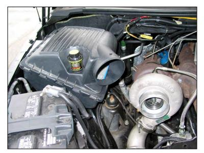
Remove the air cleaner box to turbo inlet hose.
