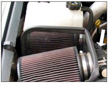
Install the airflow sensor and secure in place. Install the air inlet hose and secure with the hose clamp.
