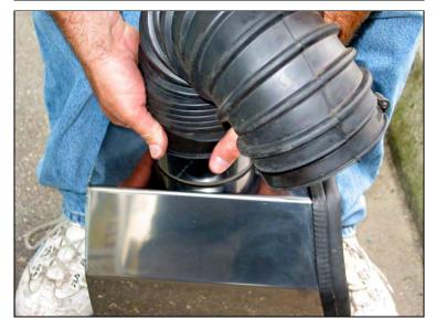
Insert the turbo inlet hose onto X-Intake Airbox housing as shown.
