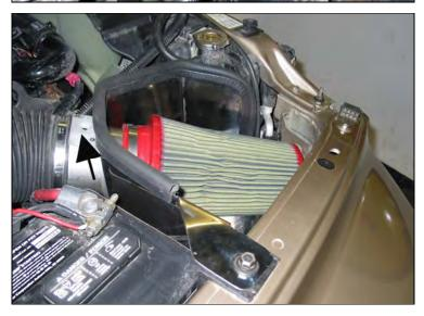
Insert the Intake Air Temperature (IAT) Sensor into the hole on top of the X-Intake airbox and refasten using the factory screws.
