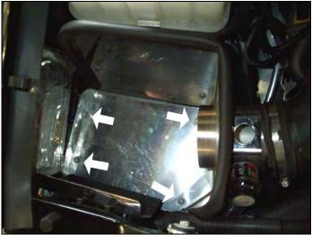
Install the X-Intake Airbox in place and secure with four (4) mounting bolts.
