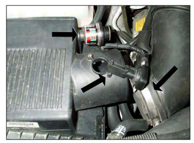
Remove the air inlet hose and airflow sensor.
