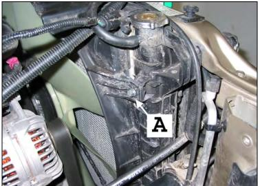
Remove the factory bolt and install the supplied Fan Shroud Support (A) bolt. Re-use the Battery Tray bolt and tighten snugly.
