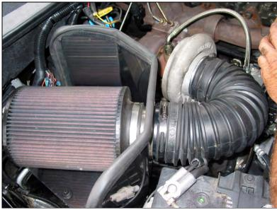
Install the air hose to the turbocharger and tighten all clamps.
