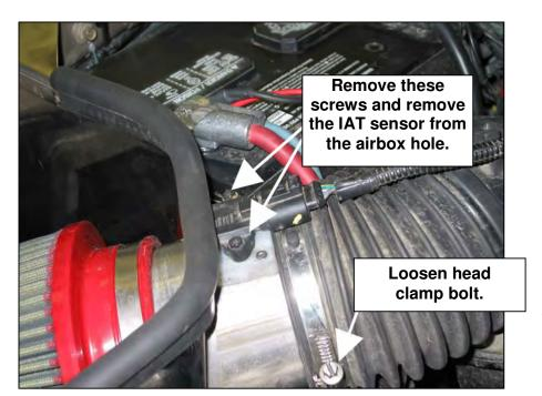
Loosen the band clamp and remove the air inlet hose from the stock airbox.
