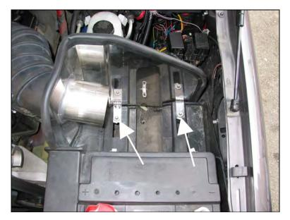
Install the X-Intake Airbox into place and secure with the two factory mounting bolts. The two bolts near the battery are **NOT** re-used.
