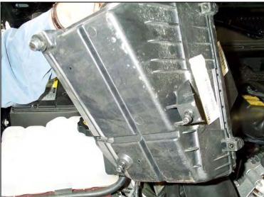
Remove the airbox from the fender well.
