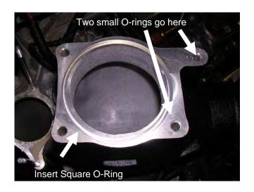
Flip the BD Intake over and insert the intake over and down through the studs until it is mounted to the factory intake plenum.
