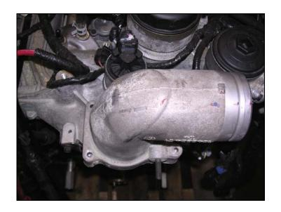
Attached to the bottom of the factory intake elbow will be a rectangular rubber seal. Store this in a safe place as it will be reused later.
