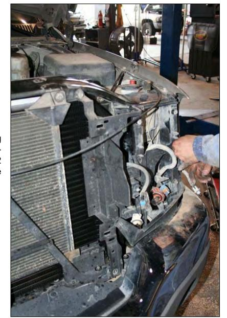
Install the two headlight mounting panels with the 6 - 10mm and 2 - T25 Torx. Make sure to put the 2 Torx in the same place they came out for proper headlight clearance.
