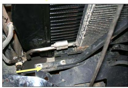
Loosen the boot clamps with a 7/16 deep socket on both the driver's and passenger side.
