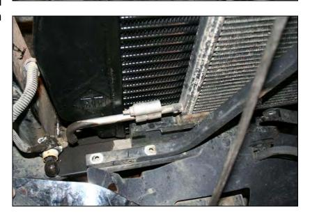
Bolt the radiator to the CAC. Use the 2 new M8 x 35mm bolts (1100035) and M8 washers (1462609) supplied and bolt the CAC to the upper tie bar.
