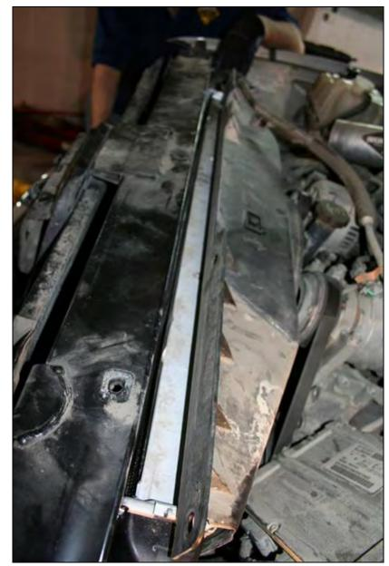
Remove the upper fan shroud. There are 2 push fasteners on each side holding it to the lower shroud and 4 - 10mm head bolts across the top to the tie bar.
