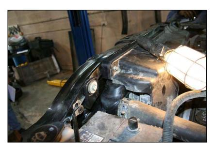
Install the upper fan shroud with the 2 push fasteners per side, holding it to the lower shroud.
