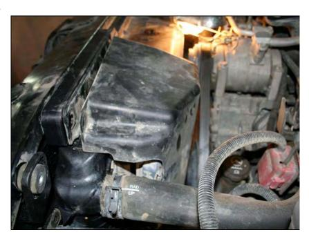
With a 10mm socket, install the hood latch with the 3 bolts taken off earlier (The position is critical, make sure it lines up to the tie bar paint pen marks).
