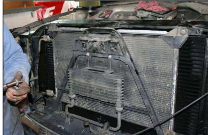
Remove the support strut from the driver's side fender to the tie bar.
