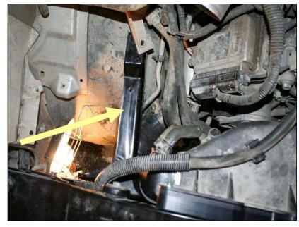
With a 10mm socket, remove the three hood latch bolts (The position is critical, mark where it lines up to the tie bar with a paint pen).
