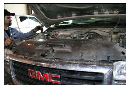
Install the radiator closure panel with the 7 push fasteners.
