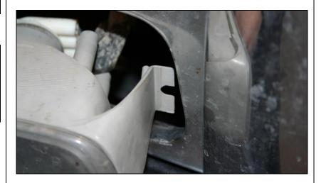
3. Remove the 1 bolt holding the grill to the Rad Support/Tie Bar Assembly with a 10mm socket. Use a clip removal or similar tool to release these clips shown here, and the far outer clips can be removed by pulling them out by hand.
