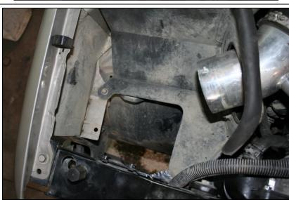
6. Remove bolt connecting coolant bottle to fender bracket (10mm), disconnect A/C line clip and then push pin from inner fender on wheel side. Loosen 2 (10mm) bolts holding bracket to rad support then lift bracket out of truck.
