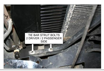
12. Carefully lift rad and CAC upward then remove CAC.
