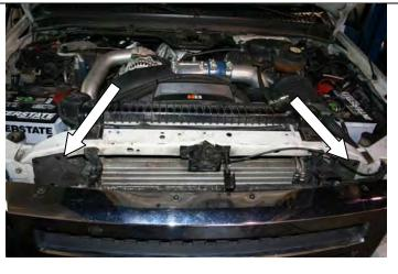
4. Mark the hood latch position with a felt or paint pen.
