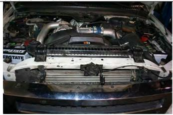
12. Mount the (1407008) 3-3 1/4" step ribbed boots on the BD intercooler and tighten the (1407030) 3 1/2" clamps until the spring is bound. (1/2" head)
