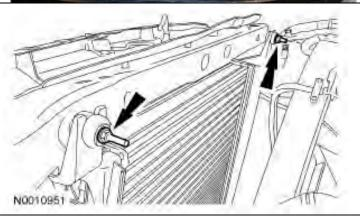
7. Lift out the top radiator support by removing 8 (13mm head) ensuring all mounting hardware has been removed.
