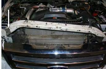
8. Move A/C condenser and lines to the passenger side to gain clearance to remove the C.A.C.
