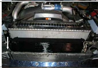
9. Switch over the top and side rubber mounting isolators from the old cooler to the BD Charge Air Cooler (1402700).
