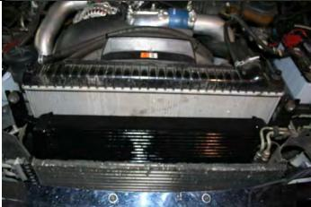
11. Reinstall the top radiator support and continue to reconnect the C.A.C. mounting bolts, top radiator mounting brackets, A/C condenser brackets and hood latch.
