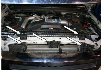
6. Locate and remove the C.A.C. bolts for the top radiator support. (10mm head)
