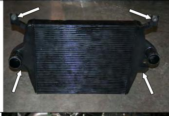
10. When positioning the new Charge Air Cooler into position move the A/C condenser and lines to the passenger side to gain clearance while seating the side isolators firmly in place.
