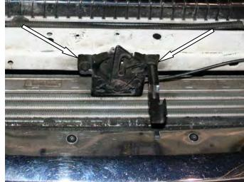
5. After you have marked the hood latch you can now remove the top radiator mount brackets, A/C condenser brackets and hood latch.
