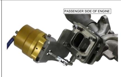
3. Insert the last four studs into the T4 side of the diverter valve and slide on the supplied T4 gasket. You are now ready for your turbo installation. Once your turbo is in place using the final 4 nuts tighten the turbo into position then torque to 35 ft/lbs.
